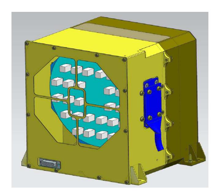
Mechanical flux **attenuator** 32 CdTe sensors on Caliste-SO hybrids Analog-to-digital converters **Data processing unit** (IDPU) Low-voltage/sensor bias **power supplies**
