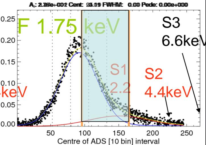
The statistical uncertainties in the number of ion-electron pairs formed and gas gain result in a *pulse amplitude distribution* where photons of constant energy are absorbed. *Detector resolution,  $\Gamma$* , (in eV) is the full width at half maximum of its pulse amplitude distribution, given empirically by
