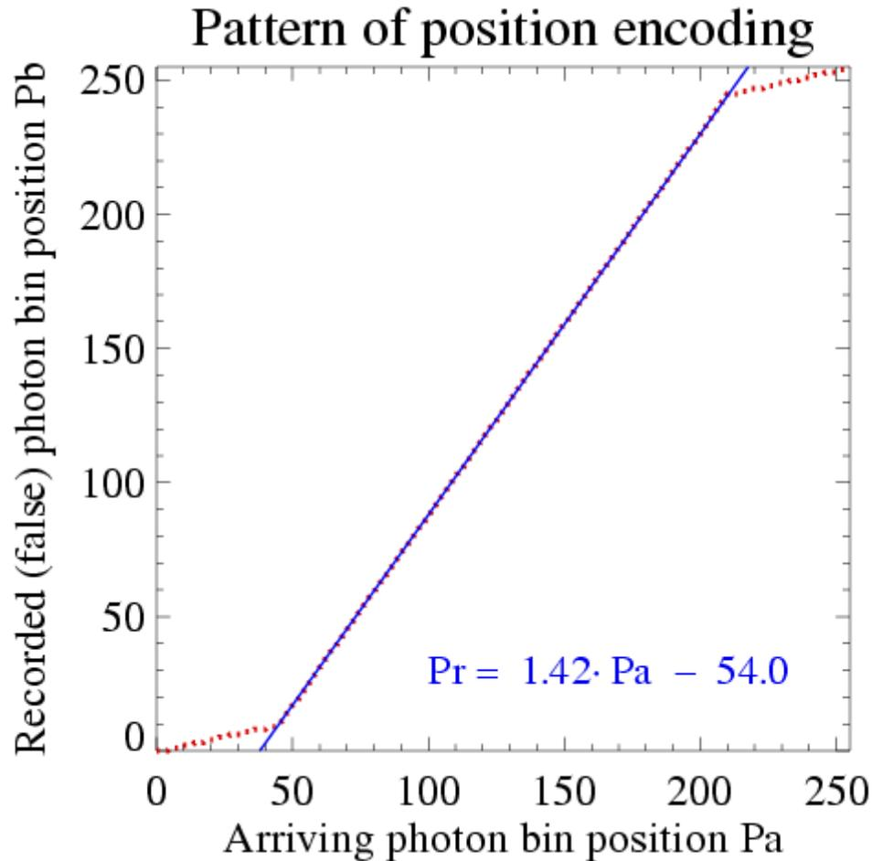
The region along the active length of the position encoding is zoomed electronically at the cost of edge, hidden bins lengths
