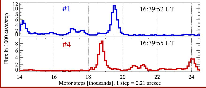
An example of measured spectra recorded nearly simultaneously in Channels #1 and #4 of Diogeness during the maximum phase of X5.3 flare on 25 Aug. 2001. The scanning in both channels is made in the opposite wavelength sense. Thus the intercombination and forbidden lines comprising the Ca XIX triplet are seen on the opposite sides of the presented range (recorded 20 s apart in time).
