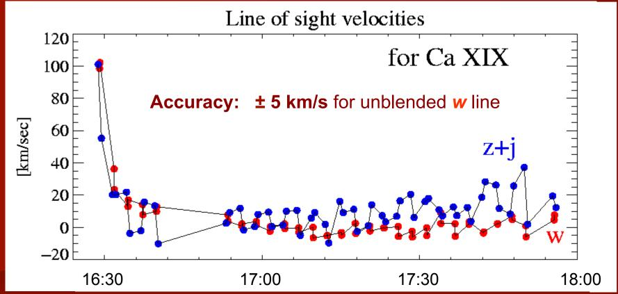
Velocities as determined for the resonance (w) and forbidden lines (z) of the Ca XIX triplet. The forbidden line is blended with a strong dielectronic satellite line (j) which might account for slightly different pattern of behaviour later in the flare decay.
