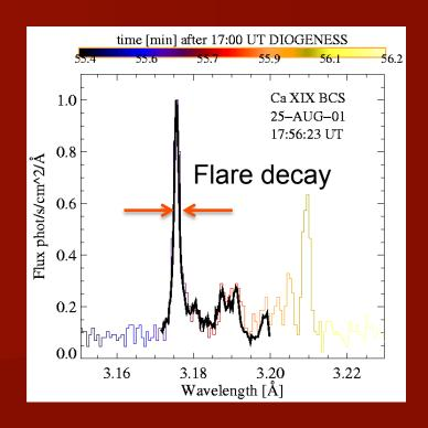
Variation in line widths is due to changing plasma turbulentce The colours correspond to times at which particular wavelength has been scanned by Diogeness. The *Yohkoh* BCS spectra have been observed close in time.
