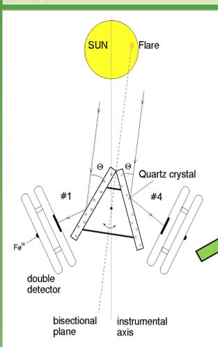
The scheme of dopplerometer section of **Diogenes**. The bi-sector plane of the pair (Q1 and Q4) of identical Quartz monocrystals (1011) points towards the X-ray source (flare). Crystals are fixed together mechanically at the exact angle of  $2\theta$ . According to the Bragg condition:
