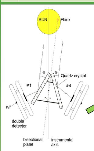
The scheme of dopplerometer section of Diogenes. The bi-sector plane of the pair (Q1 and Q4) of identical Quartz monocrystals (1011) points towards the X-ray source (flare). Crystals are fixed together mechanically at the exact angle of  $2\theta$ . According to the Bragg condition:
