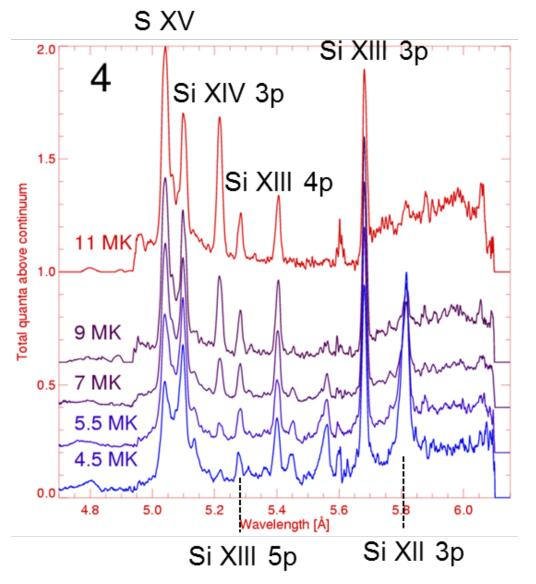
1163 RESIK spectra collected between 1 January and 14 March 2003 (best observing sequences) were grouped according to the emitting plasma temperature and averaged in order to reveal spectral features in detail. The collected set of spectra covers as well lower class events (~B4) as few M class flares. (Sylwester, B. et al., Adv. Space Res., 38, 1534, 2006)
