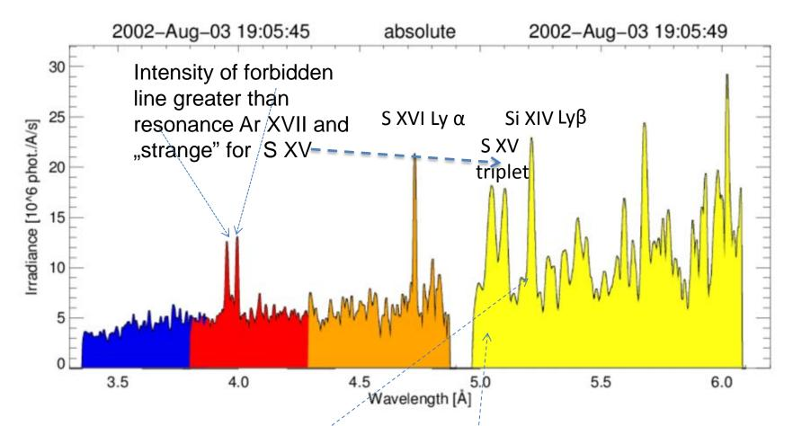
In **hot** thermal plasma, the intensities of triplet lines preserve a well known pattern with the strongest resonance transition, weaker forbidden and the weakest intercomination lines. The relative intensity of Si XIV Lyβ line exceeds the S XVI Ly α line intensity which is unusual.
