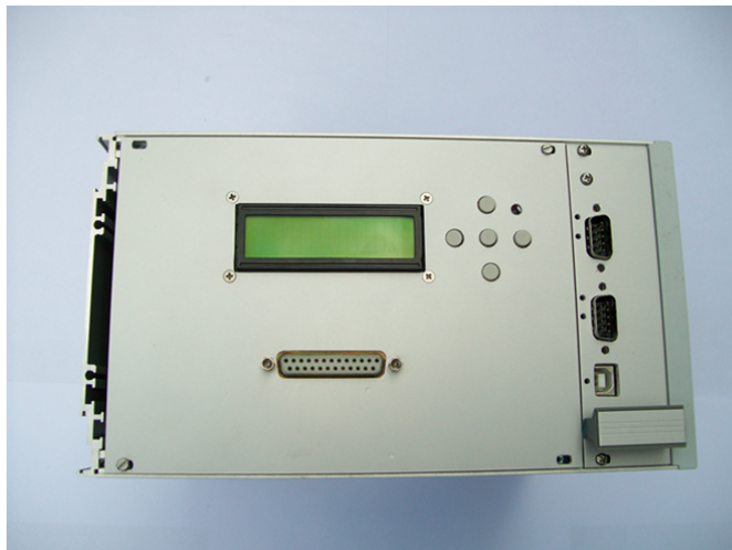
Symulator złącza SpaceWire, termoregulator (Cold Finger Simulator).
