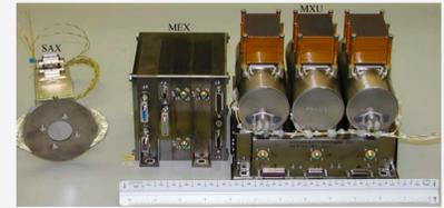
Figure 2: XRS spectrometer
