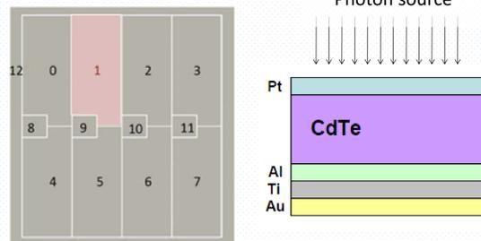
Simulations were performed assuming monoenergetic photon source with energy changing from 4 keV to 180 keV in 0.1 keV steps. The photon source was planar with a size equal to a size of CdTe sensor. Photons felt at right angle to the crystal surface and their distribution was uniform. For each energy we simulated 1 million photons.
