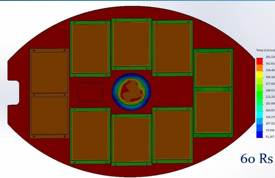
Solar Flux at distance 60Rs is 17.5KW/m<sup>2</sup>
