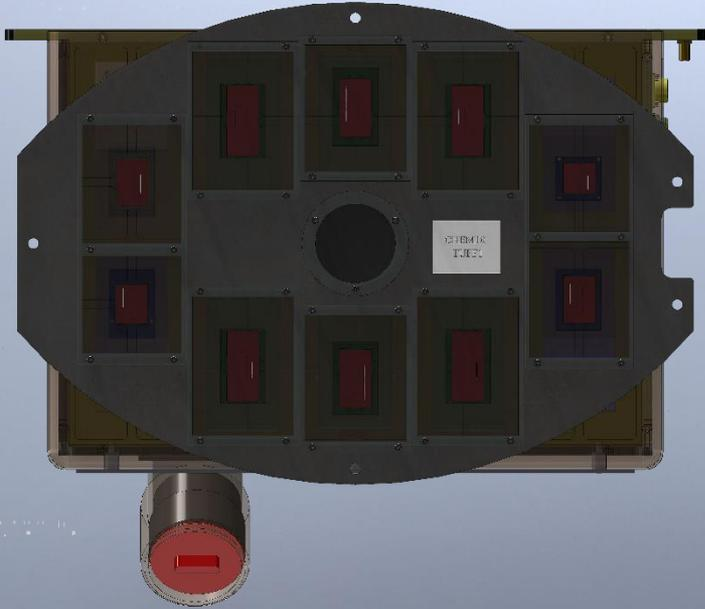
General view of the ChemiX Bragg spectrometer (right). The upper two panels are the filter boards to be mounted on the mission thermal screen. They have to withstand harsh thermal conditions (~400 C). The crystals and detectors are mounted within the block placed ~1m behind the filters. The red-capped tube is the particle detector system, under development by the Ukrainian Kharkiv group led by Dr. Dudnik.
