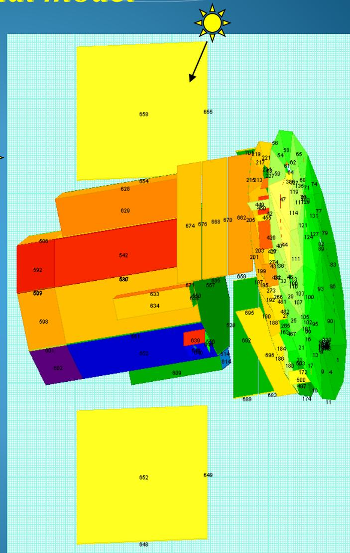
The temperature level varies widely depending on the orientation of the spacecraft ( $-100^{\circ}\text{C} \dots +450^{\circ}\text{C}$ )
