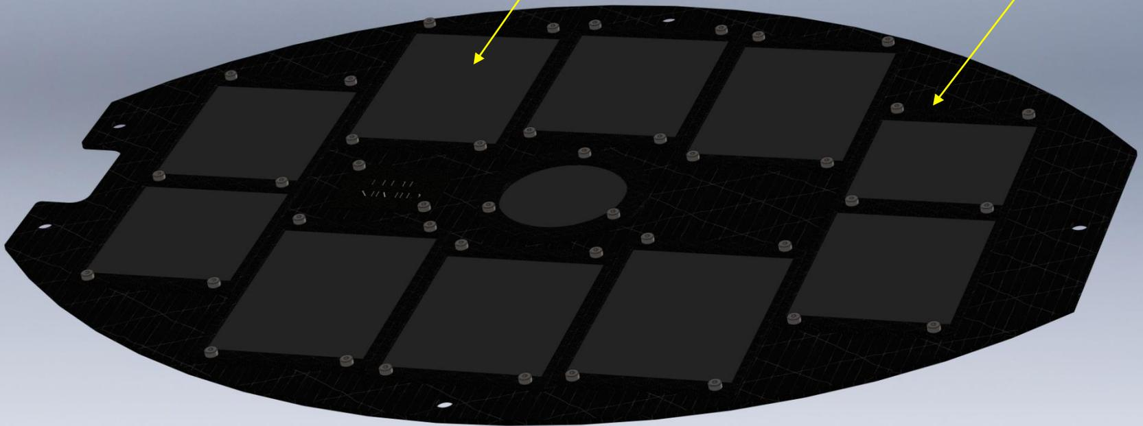
Thermal shield and X-ray filters consisting of two sections (front and rear). The main function of these two layers is to block the thermal load of solar radiation on the instrument and prevent the heat to penetrate down to the S/C.
