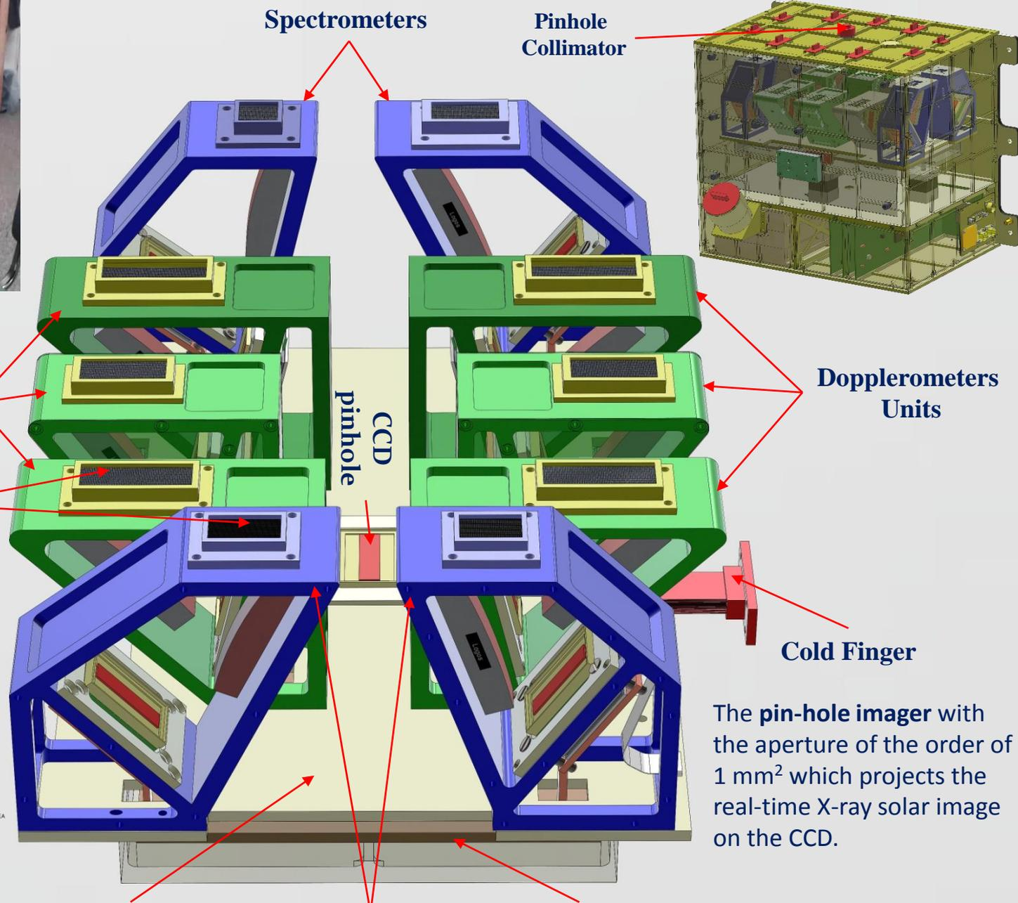
The **pin-hole imager** with the aperture of the order of 1 mm<sup>2</sup> which projects the real-time X-ray solar image on the CCD.
