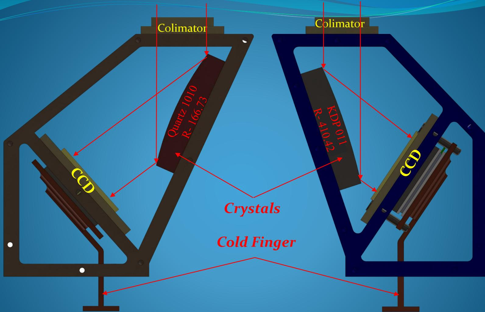
Four sections of the spectrometer cover the spectral range from approx. 1.5 Å to 9 Å
