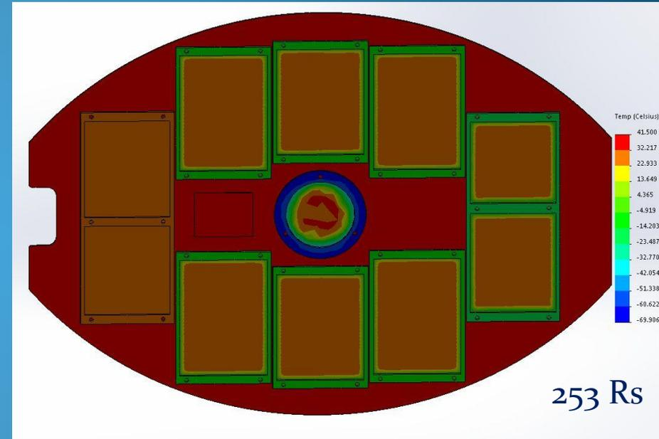
Solar Flux at distance 253Rs is 950W/m<sup>2</sup>
