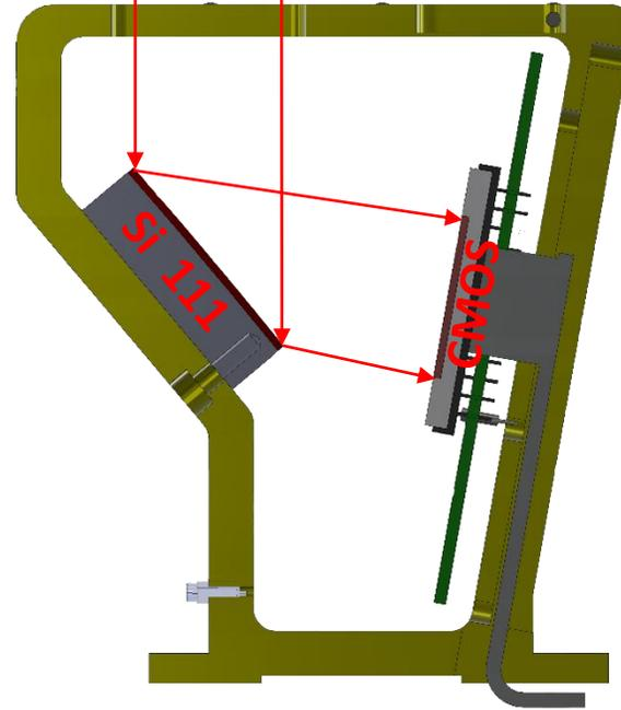
Si 111 bent crystal at the Brewster angle  $\sim 45^\circ$
