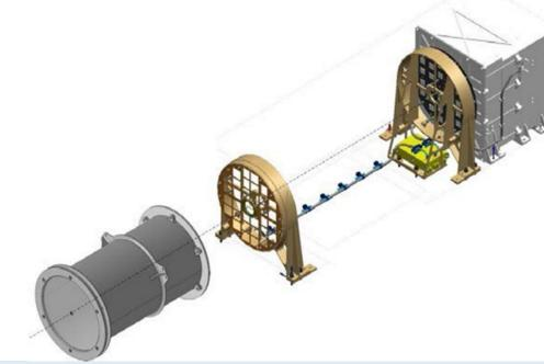
components of photon source with set of grid pairs. Each pair of grids generate a Moiré pattern and encode direction of incoming photons. Next, the pixelised CdTe semiconductor detector detect large-scale intensity distribution of the pattern, which is a Fourier component of the image. An image can be reconstructed using many such Fourier components.
