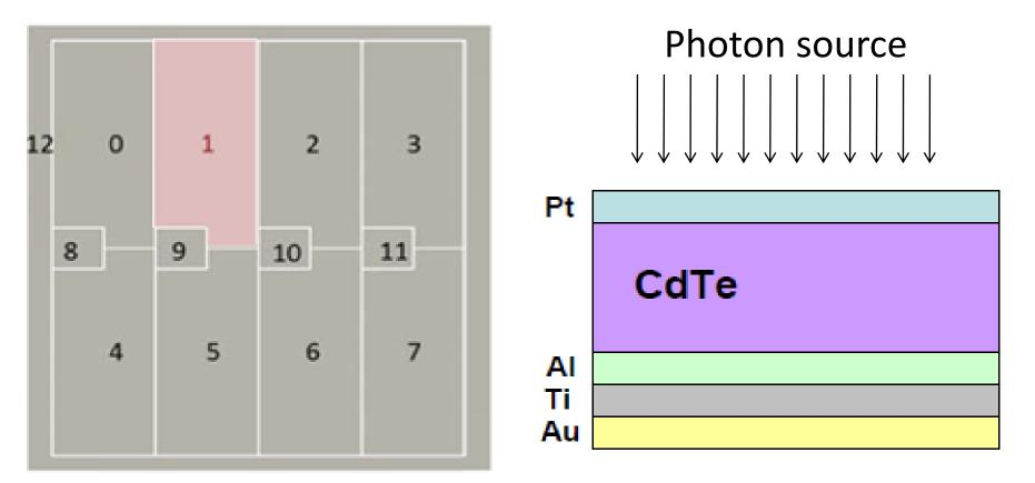
The simulated photon source was planar and cover whole detector area. Photons were monoenergetic and felt at the right angle to the crystal surface. The distribution on the surface was uniform.
