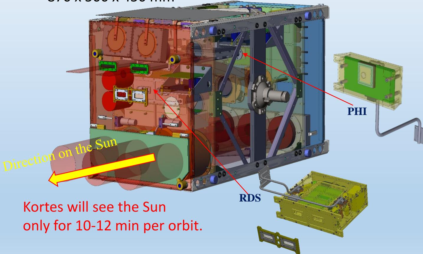
The instrument will be placed within the KORTES package. KORTES is to be placed at the top of the solar pointing platform attached to the Russian Nauka module on ISS. The pointing platform of Nauka will be guided towards the center of the solar disk.
