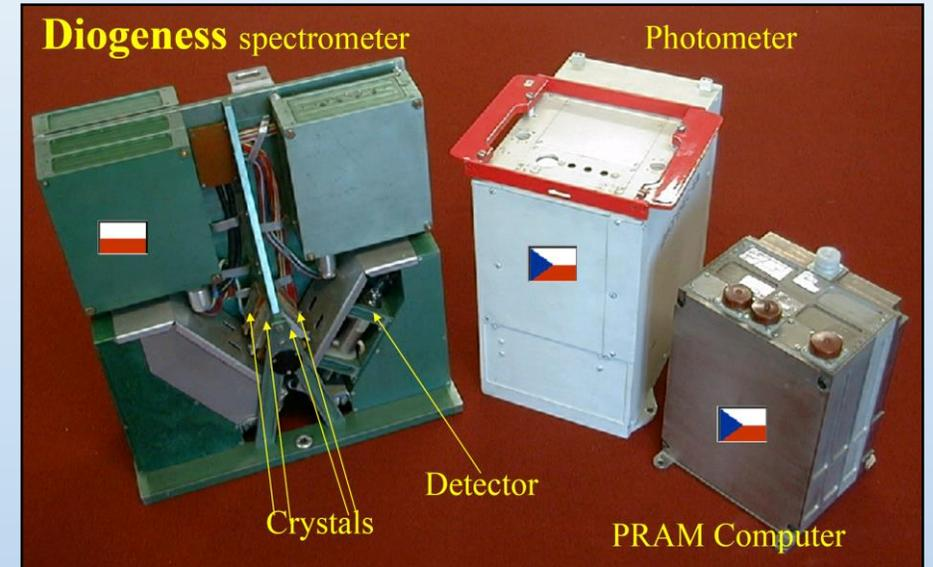
**Diogeness** was a scanning Bragg flat crystal spectrometer equipped with four mono-crystals used as dispersion elements. Two of them are identical quartz crystals mounted on the common shaft in an unique, so-called Dopplerometer configuration.
