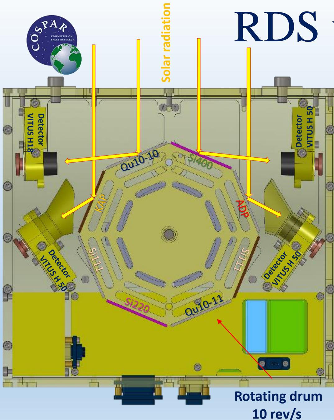
**Rotating Drum Spectrometer** contains
