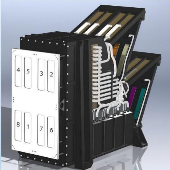
CAD illustration of the SMM Bent Crystal Spectrometer with channel numbers indicated.
