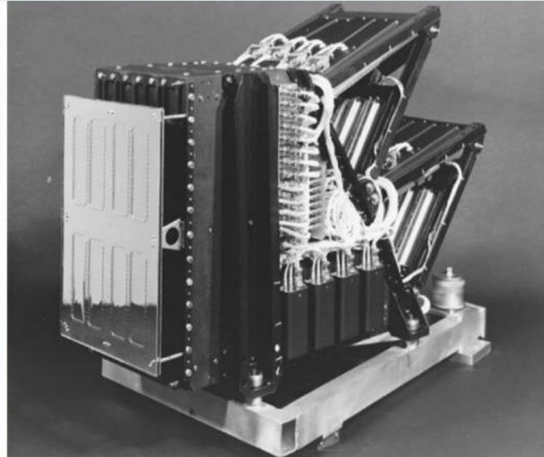
The instrument bolted to a calibration stand before installation in the SMM spacecraft.
