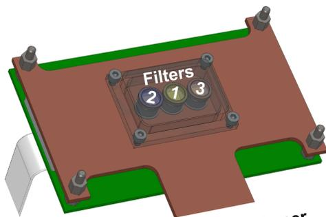
Three Pyroelectric Laser Detectors Model 420
