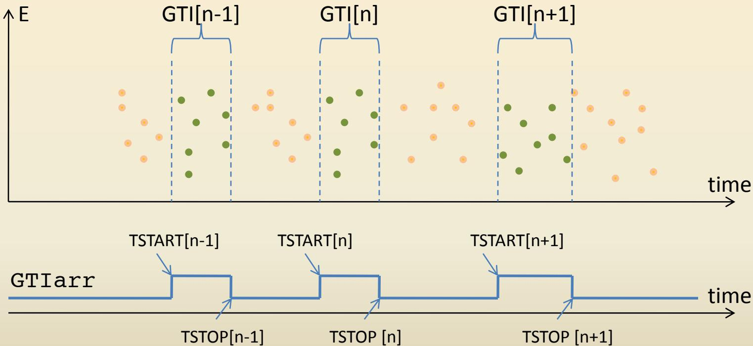
Finally we can determine TSTART and TSTOP for each GTI by edge detection in GTIarr.
