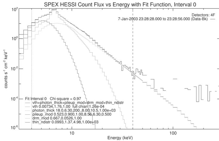
Figure 3. An example of RHESSI fit including the thin-target bremsstrahlung radiation from n-distribution. The fitting range is 4-40 keV.
