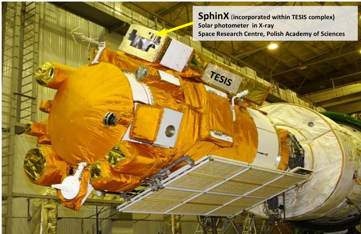
Figure 1. The *CORONAS-Photon* satellite on a top the Cyclone-3M buster placed horizontally. Locations of SphinX (within TESIS) and STEP –F (charged particles monitor) are indicated in the picture.
