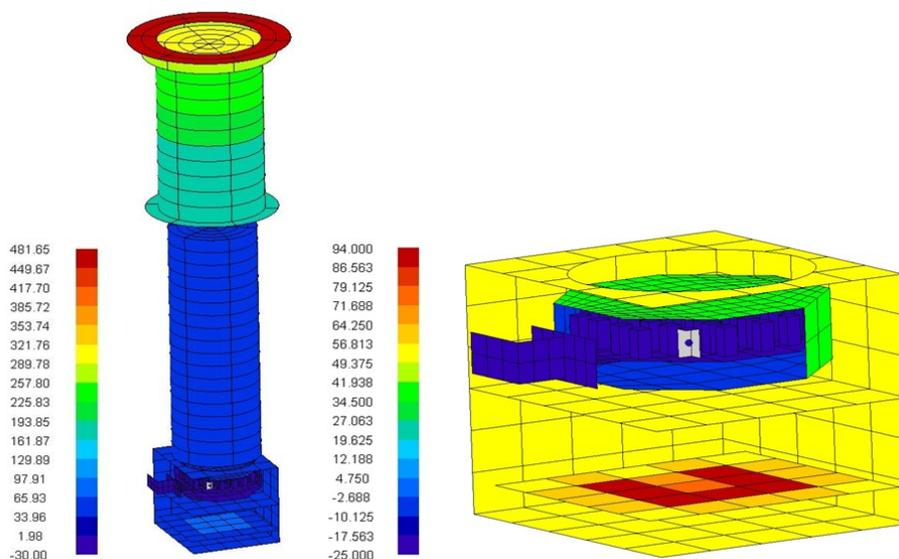
Figure 3. The temperature profiles of the STIX instrument in the hot operational case. On the right the Detectors Electronics Module is presented.
