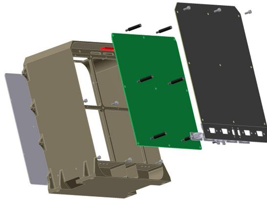
Figure 9. Mechanical enclosure of IDPU and PSU.
