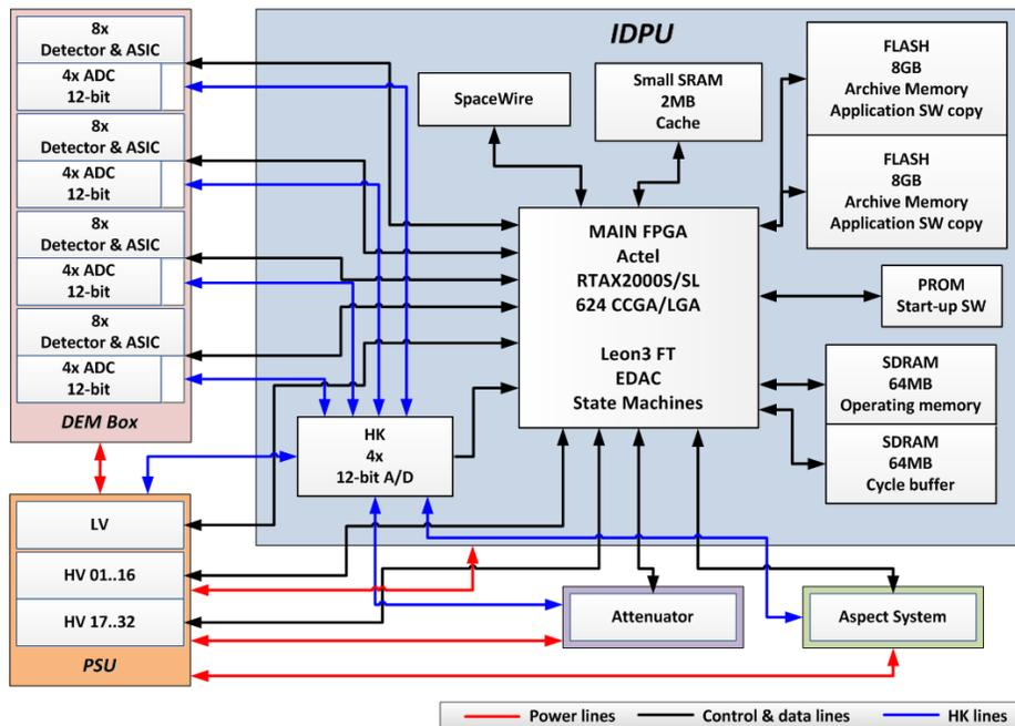
Figure 8. Logical block diagram of IDPU.
