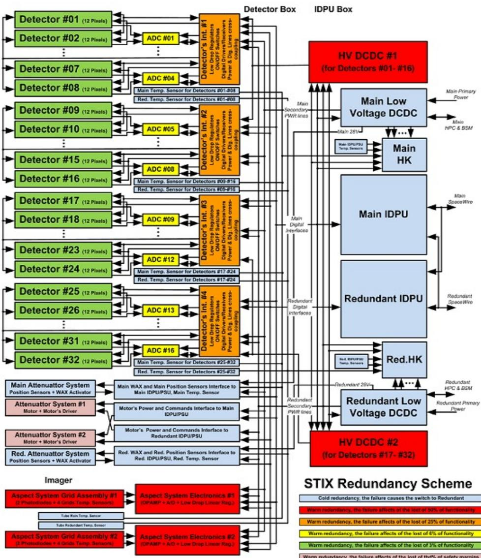
Figure 13. Redundancy concept of STIX and IDPU.
