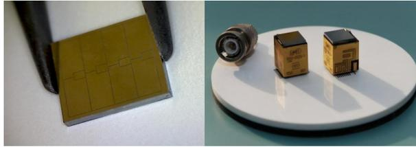
Figure 7. *Left:* CdTe detector used in STIX. *Right:* Caliste-SO spectrometer units.
