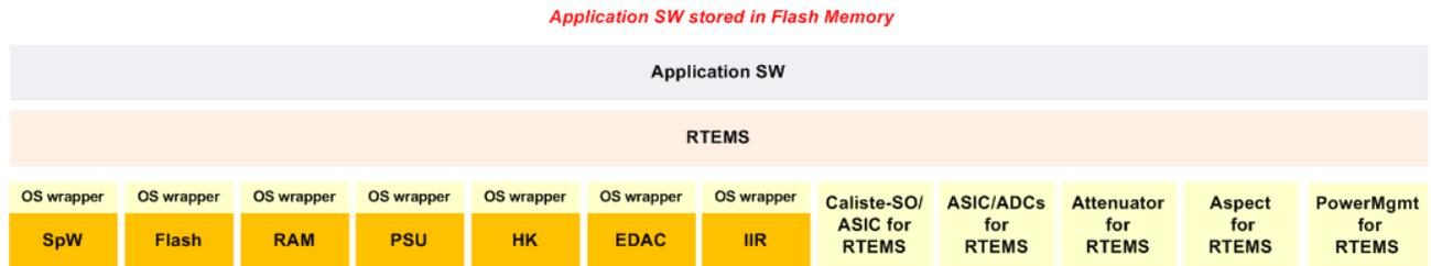
Figure 11. Basic Software drivers for Application Software.
