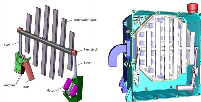
Figure 6. *Left*: Attenuator components. *Right*: Attenuator mounted on DEM Box seen from top.
