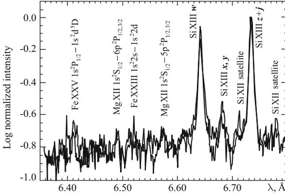
**Fig. 6** Two averaged X-ray flare spectra (two almost coinciding *curves*) of August 25, 2001 flare, obtained by DIOGENESS spectrometer in course of scanning in opposite spectral directions. The identification of principal lines in 6.35–6.80 Å range has been performed. From [5]
