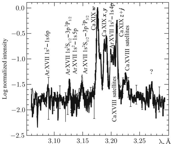
**Fig. 5** Averaged flare spectrum of August 25, 2001 flare, obtained by DIOGENESS spectrometer in the 4.98–5.26 Å range (shown, there are two well coinciding spectra averaged separately for the scans taken in two opposite directions). The spectrum covers the lines corresponding to indicated transitions. From [5]
