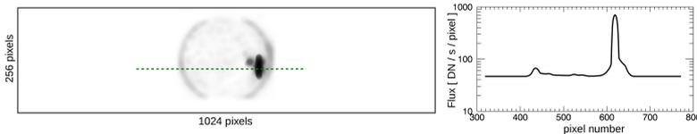
**Figure 2.** Simulated image of X-ray Sun with C5 class flare in progress projected on the pinhole camera CCD (left). The signal profile “observed” along the dashed line cut is shown to the right.
