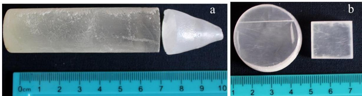
Figure 2. An ingot of the *p*-terphenyl single crystal grown by the Bridgman method (a); a cylindrical workpiece of the *p*-terphenyl with the crystallographic axes direction marking, and the *p*-terphenyl single crystal in a parallelogram form after mechanical treatment.
