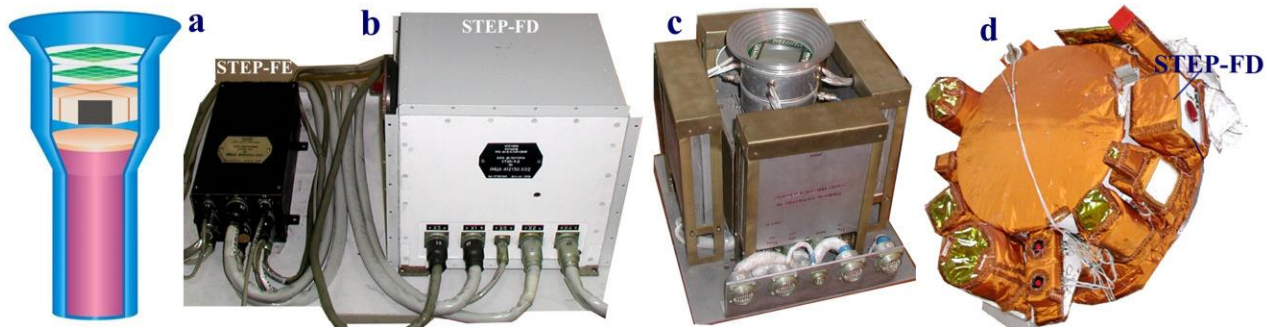
Figure 1. A structural scheme of the detector head (a); the flight (b) and the breadboard (c) models of the STEP-F; the STEP-FD unit is among external detectors of the CORONAS-Photon satellite.
