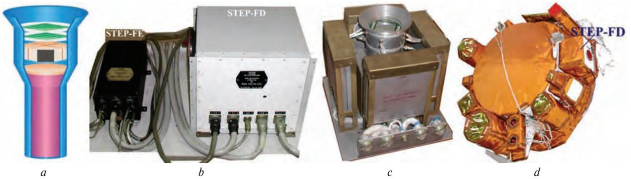
**Fig. 1.** A structural scheme of the detector head (a); the flight (b) and the breadboard (c) models of the STEP-F; the STEP-FD unit is among external detectors of the CORONAS-Photon satellite, as seen during vacuum tests (d)
