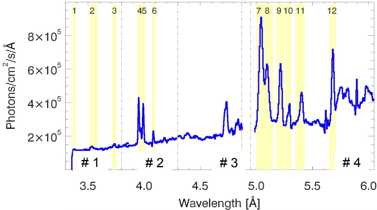
Average RESIK spectrum (integrated over 24). The dashed lines limit the four RESIK channels bands. Unfortunately, due to technical problems during this flare, channel 3 data are not reliable for the analysis for DEM calculations.
