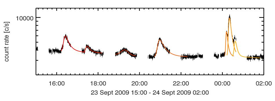
SphinX 1.2 - 10 keV lightcurve with optimal fit of elementary flares.
