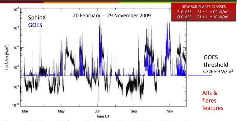
Figure 1. Solar fluxes in 1-8 Å energy band calculated from SphinX data (black colour) compared with those observed by GOES (blue colour). The characteristic features of ARs and flares can be seen. It is also apparent that due to lack of sensitivity GOES did not observe any X-ray flux variability below  $3.73 \times 10^{-9}$  [W/m<sup>2</sup>].
