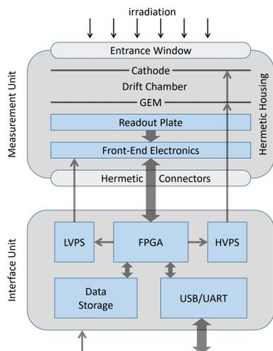
Figure 2. Block diagram of MGEM detector.
