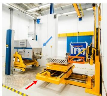
Figure 4. Underground industrial accelerator station at NDT Lab. The blue arrow points to LINAC. The red arrow points to the positioning table which has maximum load of 5t.
