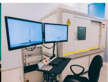
Figure 6. X-ray tomograph and its control center at NDT Lab.
