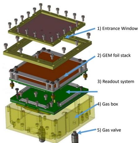
Figure 3. Exploded CAD drawing of the MGEM detector. Interface unit is not shown here. After integration of the detector all components 1), 2) 3) will be placed inside the gas box 4) and gas valves 5) assembled to it.
